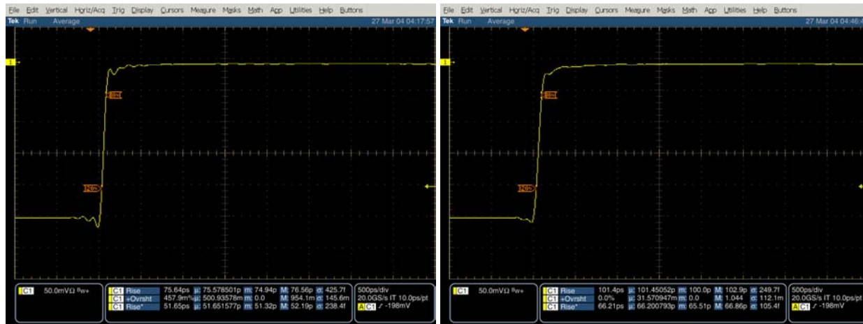
Figure 3. Step response of TDS6804B illustrates accuracy of risetime measurements. The display at left shows 76.64 ps risetime measurement from the 75ps hw filter DUT. The display on the right shows a 101.4 ps risetime measurement on the 100 ps external hw filter DUT. Use of ET mode rather than IT mode would have further reduced error in this measurement.
