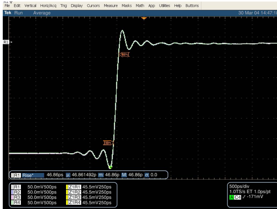
Figure 6. All four channels overlaid with B_w+ turned on and deskew adjustment made to time align. Risetime readout using 10% to 90% is 46.86 ps using a 15.5 ps step generator. An average of 500 was used.
